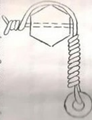
DOUBLE TWIST METHOD - CORRECT
