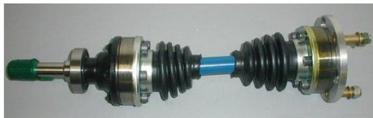
Another interesting variant is that provided by RD Enterprises of the USA. Their solution is to integrate an uprated differential output shaft into the drive line, rather than retaining what becomes a redundant joint between the output shaft and first CV joint. This solution has a good number of supporters in the US, as well as some in Europe. JAE of the US also provide a solid shaft alternative, similar to the Kelsport offering.
