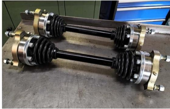
More recently onto the market is Australian firm Elantrickbits. They have developed solid billet axle shafts, CNC machined from high-grade alloy steel. In addition they fit grease nipples for easier lubrication and also claim that their shaft will operate through the Elan's steeper drive angles without locking up. They use the GKN CV joints and a unique to them adapter plate.
