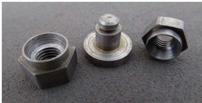
New pulley wheel post and riveting nuts
