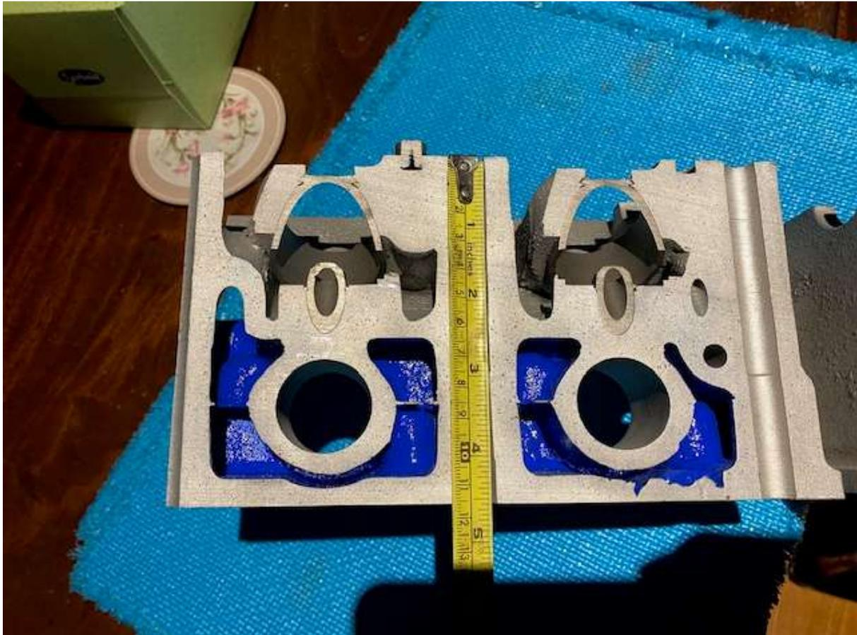
When heads have had a lot machined off the bottom face to restore flatness then the top face may also have been machined and the cam bores re-machined to restore straightness also. All these dimensional changes due to historical maintenance machining can make building a modified head more challenging which makes starting with as close to original head as possible, desirable.
