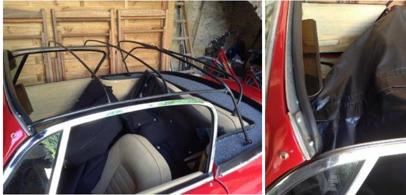
The neat arrangement of the Classic Transport Company roof mechanism and the windscreen header
