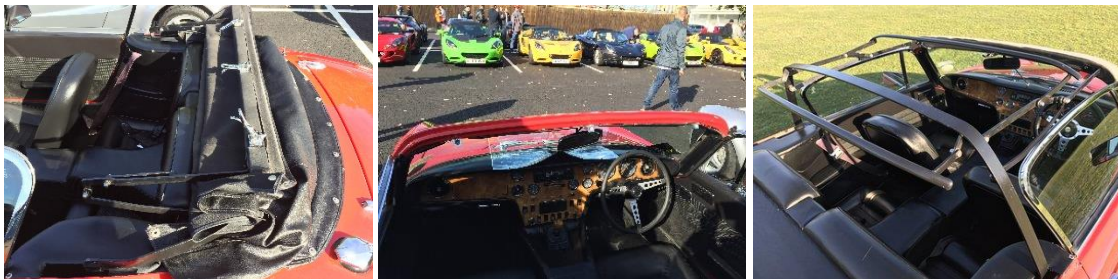
The Hexagon folding roof mechanism exposed
