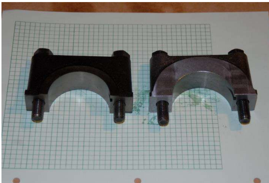
Ford square cast main caps as supplied with the new Ford Motorsport 711M blocks. Note the machining for the full circle thrust bearing on the centre cap on the right
