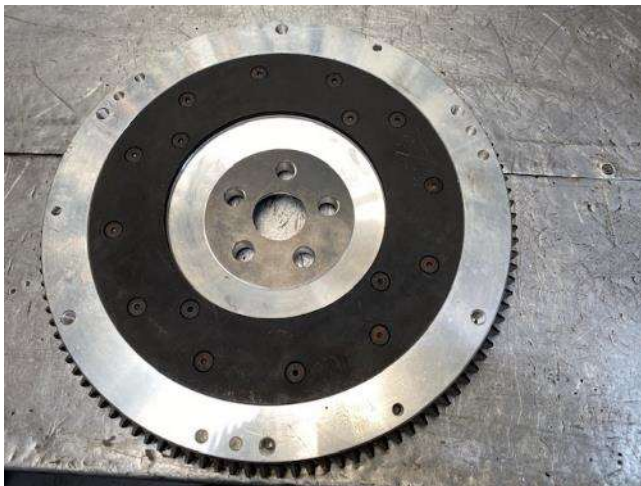
Aluminium flywheel with steel insert wearing surface for clutch plate, weight is 3.6 Kg about half that of the standard cast iron flywheel. Note also the large, hardened steel 5 bolt hole “washer” for the crank bolts to stop them sinking into the aluminium. This is for the 5 bolt Datsun steel crank in my Elan.
