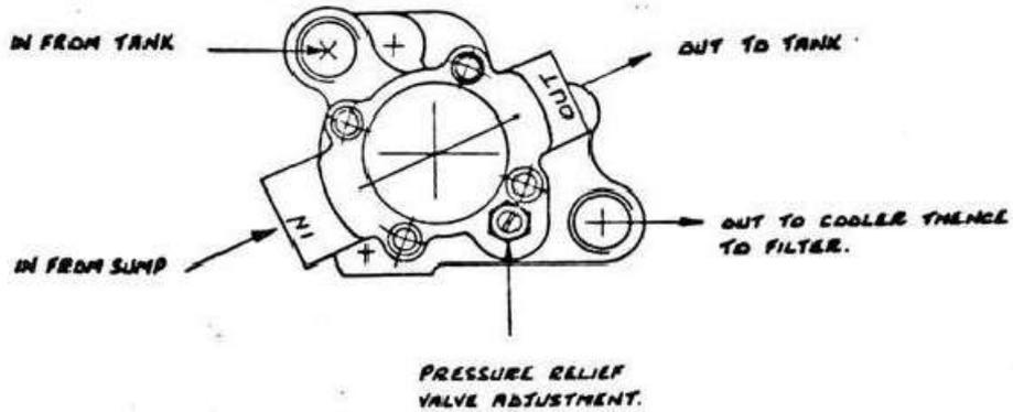
DIAGRAMMATIC VIEW ON SIDE OF ENGINE
