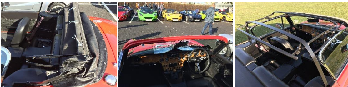
The Hexagon folding roof mechanism exposed
