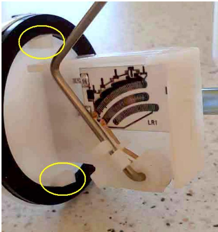
Showing the standard spade in an insulator for the green/black gauge wire, and the under-sized earth wire spade riveted directly to the base.
