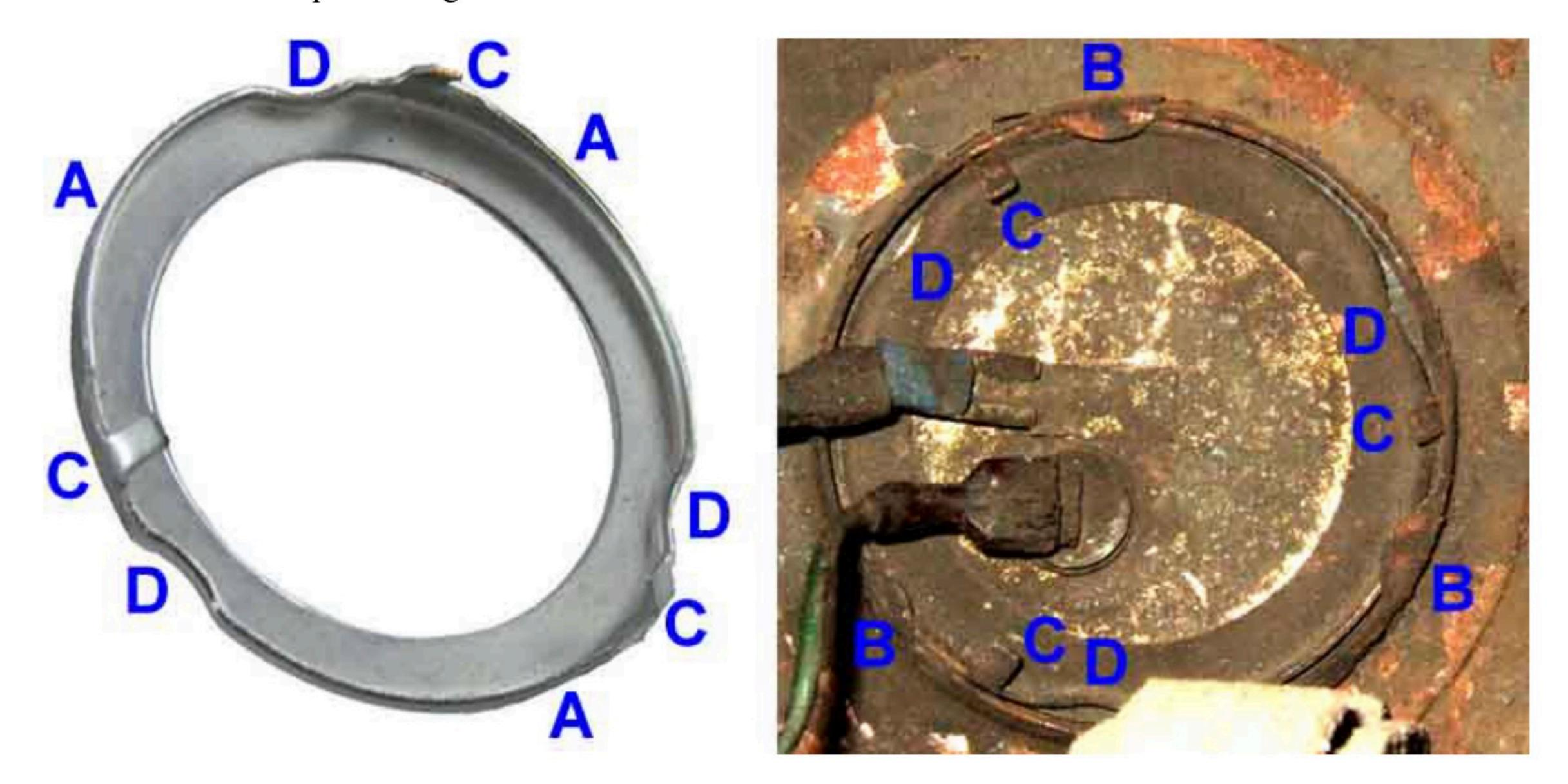
If the three tabs 'C' have been sheared off (as happened to Mark Morris) you will have to try something else. One possibility is to carefully drive the locking ring in at least two of the recesses 'D' and use self-tappers with the points ground down once the thread has been started. If you lead points on they could dig into the tank part of the fitting and you will be no better off.
