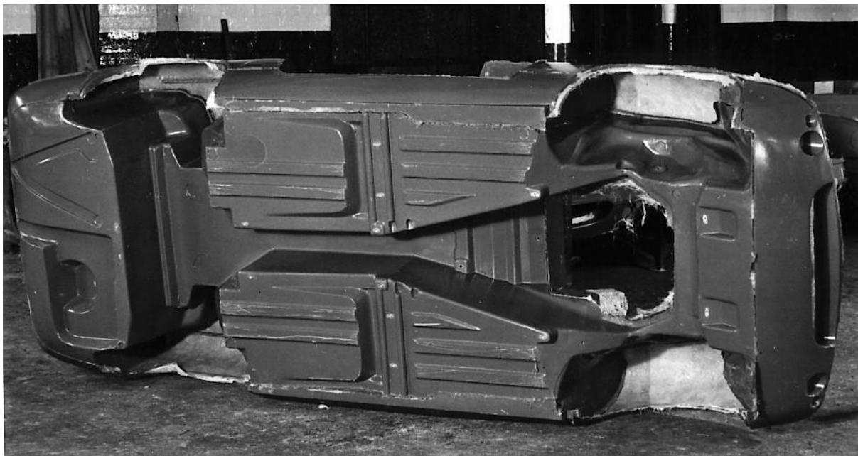
The underside of the bottom body mould, showing the strengthening ribs in the floor panels
