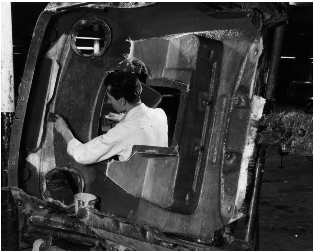
In what today would be termed a challenging health and safety environment, chopped strand matt is resin-ed into the front of an Elan
