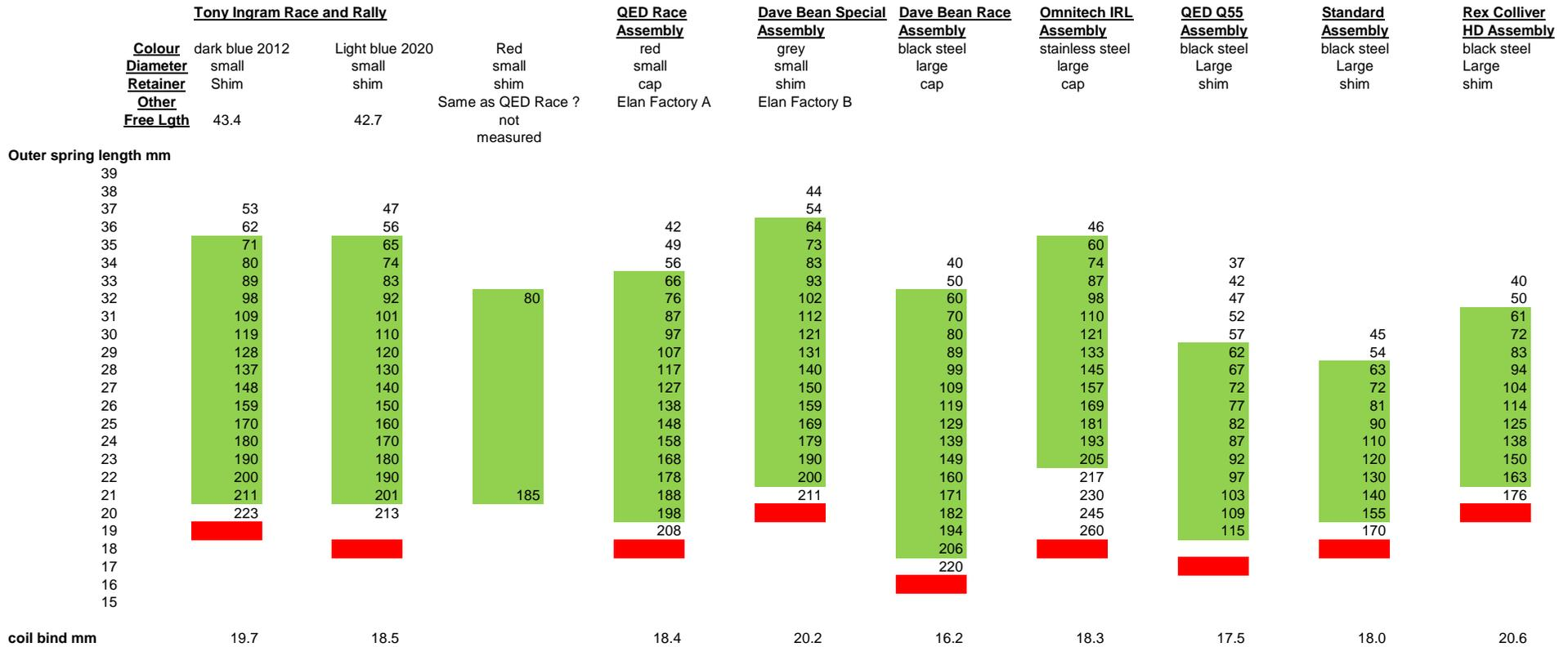
**Notes** Green region acceptable load for seat at > 60 lbs and nose at < 210 and coil bind clearance on nose >1.5mm
