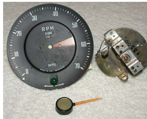
Removing needle and disassembled gauge.
