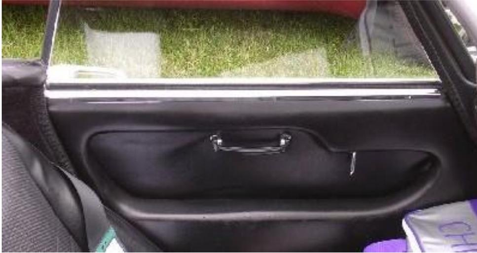
*The SS door panel with suspended handle and revised door pull*
