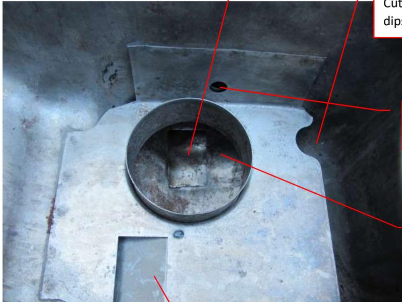
Swinging gate. Normally open for oil drain back. Closes when struck by oil from underside
