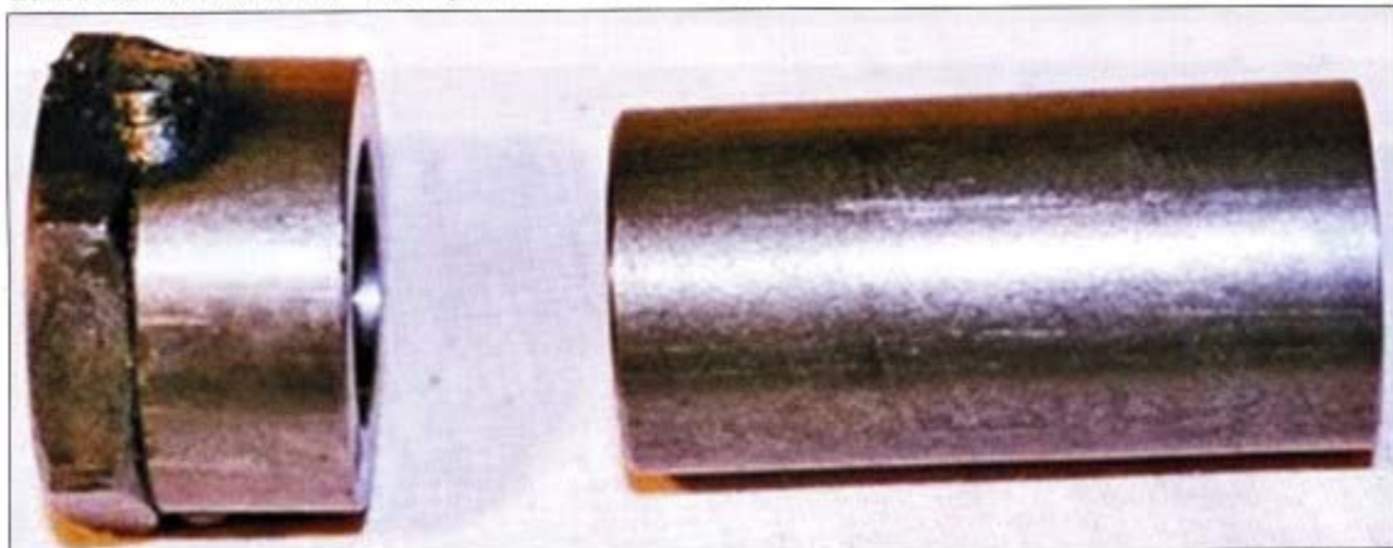
ELAN S4 AND SPRINT LOCK RESTRICTORS. YOU CAN CLEARLY SEE THE LOCKNUT WELDED TO THE SPACER FOR THE PINION SIDE. THE PASSENGER SIDE IS A MACHINED TUBE WHICH EXACTLY MATCHES THE RACK TUBE AND JUST FLOATS ON THE RACK
