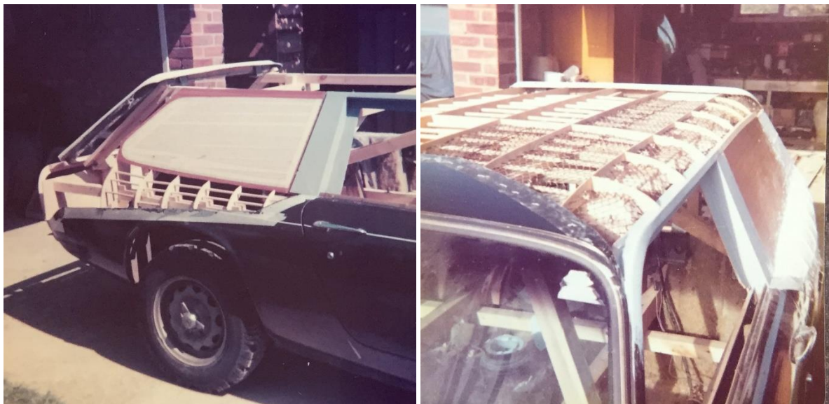
The rear side window area was formed using ply and dowels, the roof line being built up with wood framing and chicken wire, in preparation for mould forming, as below
