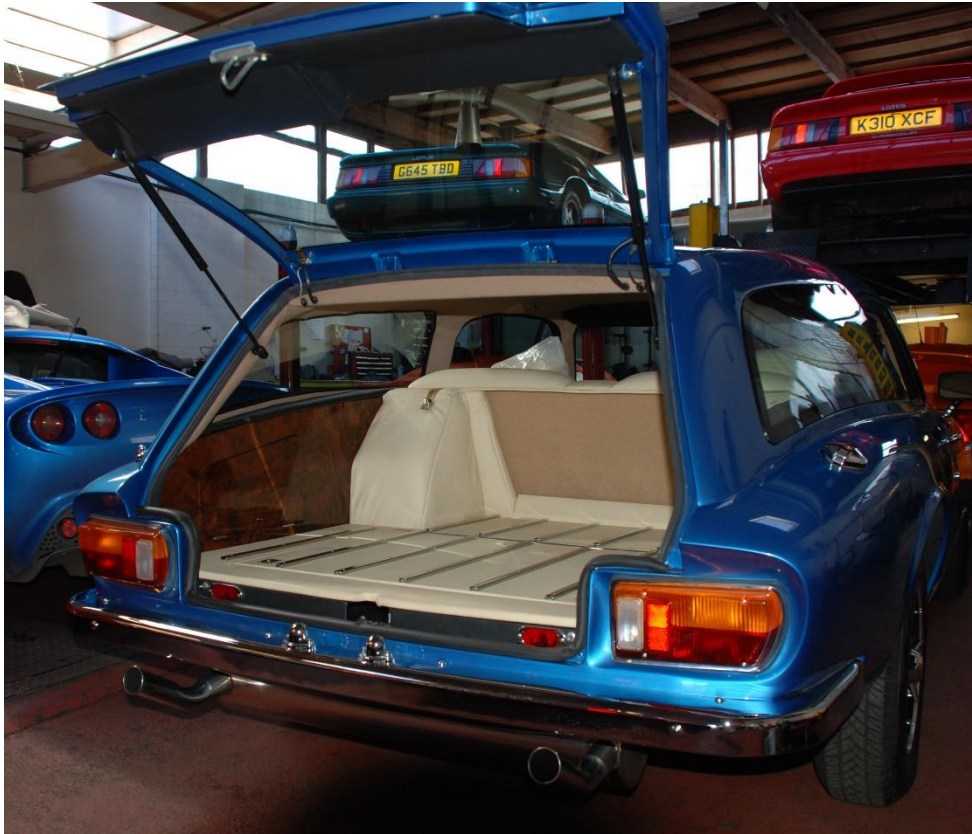
The rear load area, showing the burr walnut cubby holes, leather floor and red door open warning lights, as well as the special bespoke twin pipe silencer
