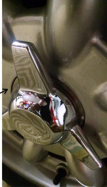
This is a similar wheel on a Lotus Elan...Note that Bushing is proud of wheel and therefore allows Spinner or Hex Nut & Spanner to clear wheel spokes.
