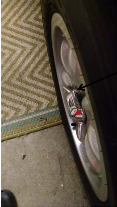
The Bushing does not put the back of the Spinner out far enough from the Spokes
