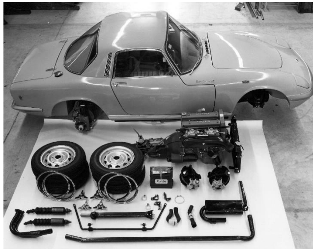
1967 S3 SE FHC in component form; this one has the rear suspension already in place
