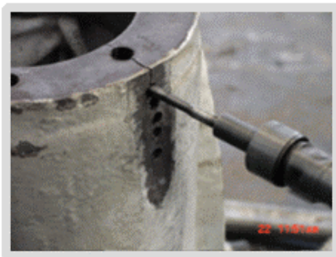
Metal Stitching with Castmaster® Pins
