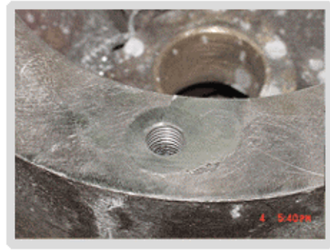
A2) Repairs with Full-Torque inserts and Castmaster pins
