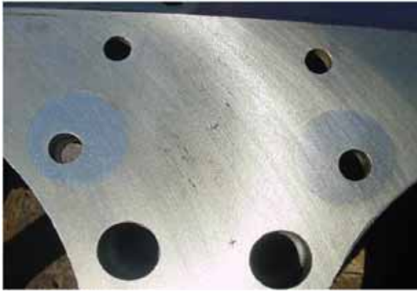
3516 Cat block with eroded water holes repaired on the deck surface. FPS plugs are installed and new water holes are drilled through the plugs
