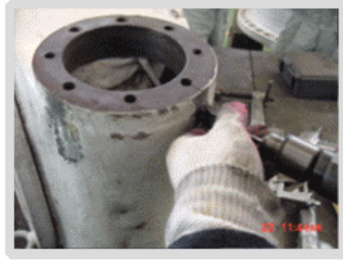
Cracked Bolt Hole
