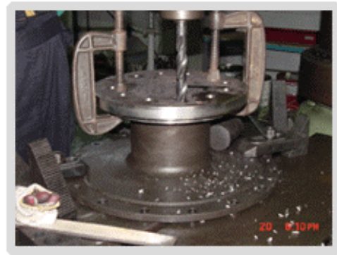
B4) Drilling of Holes
