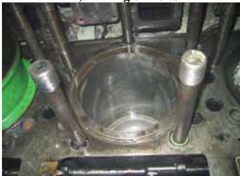
D) Installation of stud bolt with our Spiralhook thread design (For situation when our insert is unable to be install due to insufficient wall thickness to accommodate our insert)
