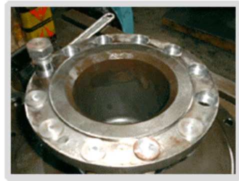
B2) Plugging of all bolt holes with our FPS style plugs
