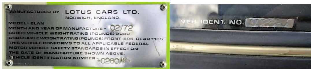
Federal conformation plate, found on the driver's side door jamb
