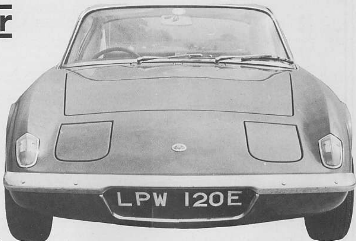
Even cleaner frontal treatment features contoured integral side lights and flashers and a steel bumper
