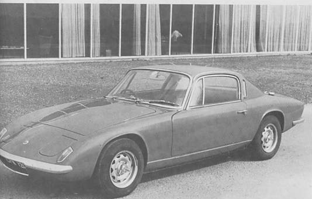
Almost 2 ft. longer and 1 ft. wider but only 1 in. higher than the Elan, the +2 has much more elegant proportions but origins remain clearly evident from any angle.
