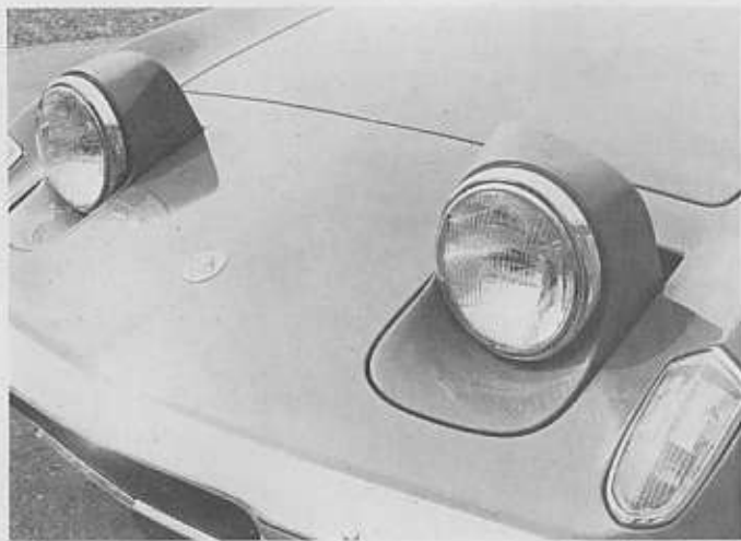
The pop-up lights, the most characteristic feature of the Elan, sprout from a flat section of the bonnet on the +2 which gives the mouldings a more angular, asymmetric form less shapely than the Elan. In daylight they emerge flashing.
