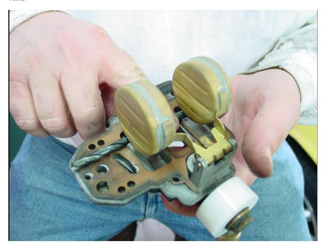
Make sure the float pivot pin is not worn and it fits into the float without any play. Yet loose enough so when the floats are tilted so the pin is vertical, the pin will fall out from gravity. When bending the tab with needle-nose pliers be careful to not destroy the extremely delicate needle.
