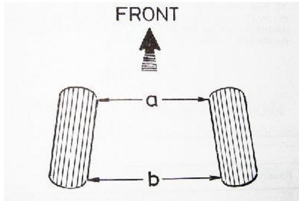
Let's assume that the toe-in is defined in mm as  $d_{toe-in} = (b - a)$  in the drawing above
