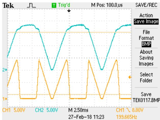
Blue shows the rectified but unsmoothed output of the battery charger. While the Yellow waveform shows FET switching waveform on the d terminal of the FET. Each waveform is 5V /division and the time base is 2.5mS/div so there is 1 pulse per 10mS or 100pps from the 50Hz mains
