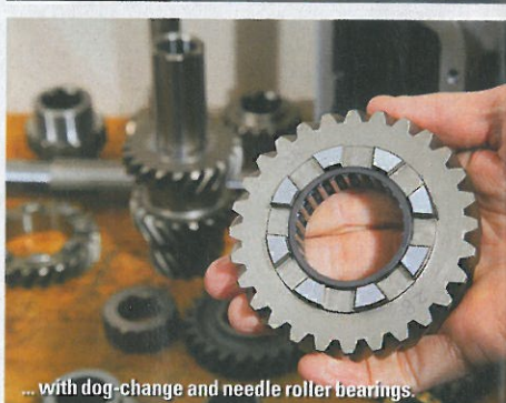
...with dog-change and needle roller bearings.
