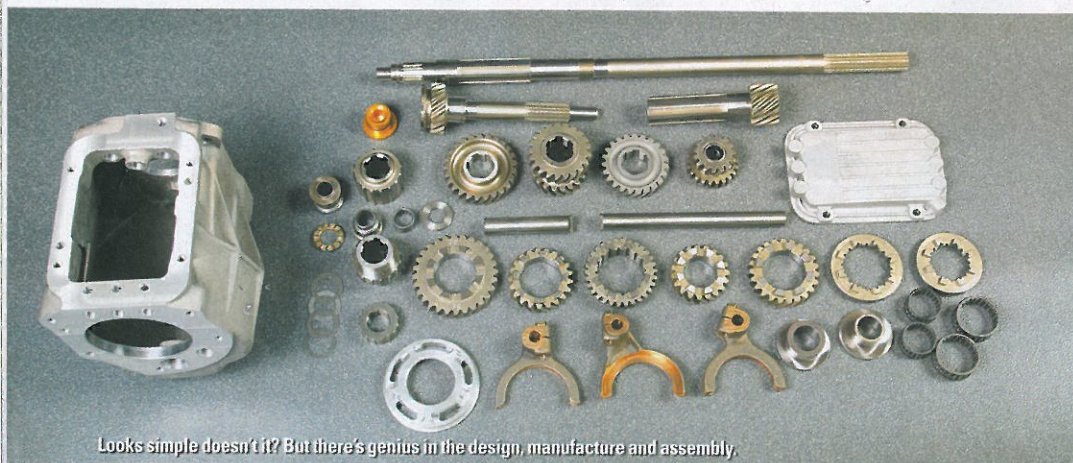
All gears used are helical cut...
