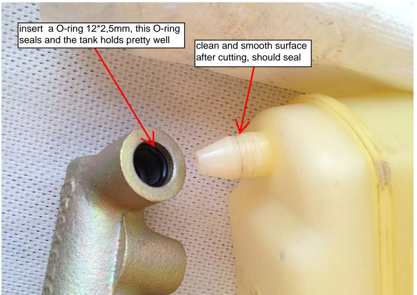
insert a O-ring 12\*2,5mm, this O-ring seals and the tank holds pretty well
