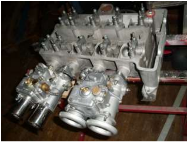
Type 1 head showing the square reinforcing blocks on the front 2 inlets.
