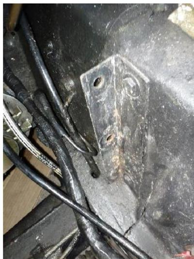
I suppose one could make cutouts to drop the radiator a bit further. Note as well that wiring and vacuum tubes need to be dressed a little to not foul the bottom of the radiator and the fibreglass lip. The access of the bottom fixing bolts are awkward - socket extensions and angle thingies would help here:
