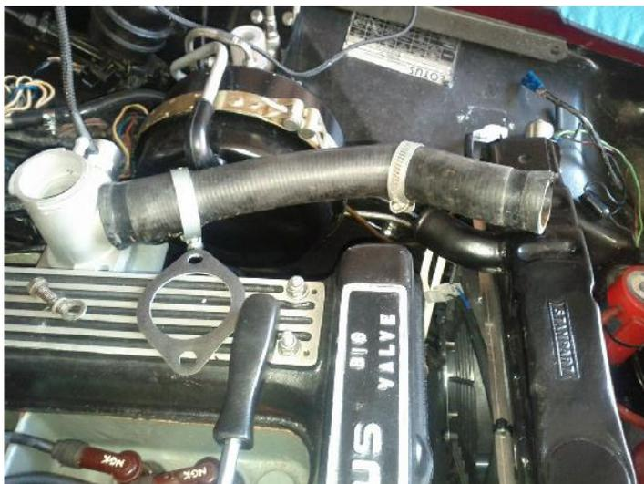
The EFC wiring unfortunately exits directly under the overflow nipple - don't like bending cables 90°.
