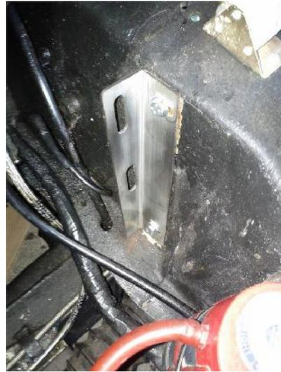
Fitting the new radiator behind the brackets left next to no room between the engine and rear-mounted fans, so I installed from the front. Still not much daylight but acceptable :
