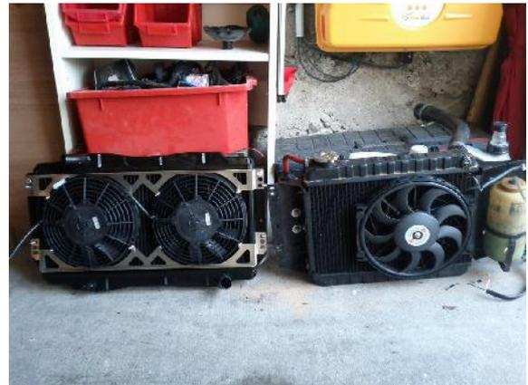
Not too many problems getting the old out - just the drain valve that was stuck ; had to spanner the whole thing out. The old brackets were a bit rusted in but they came out. Here's the old and new :
