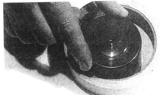
ABOVE RIGHT Chapman helped his team to understand the effect by demonstrating with a roll of tape as shown. When the cap is moved with a clockwise circular movement (not rotated) within the tape, it represents the tubular part of the traditional 'Rudge' wheel. The tape (the nut) will turn clockwise as well.
