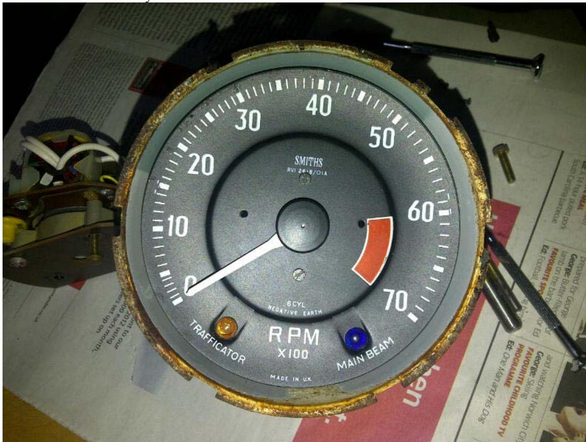
Only thing left to do is refit the diffuser ring, glass and bezel then refit to the car.
