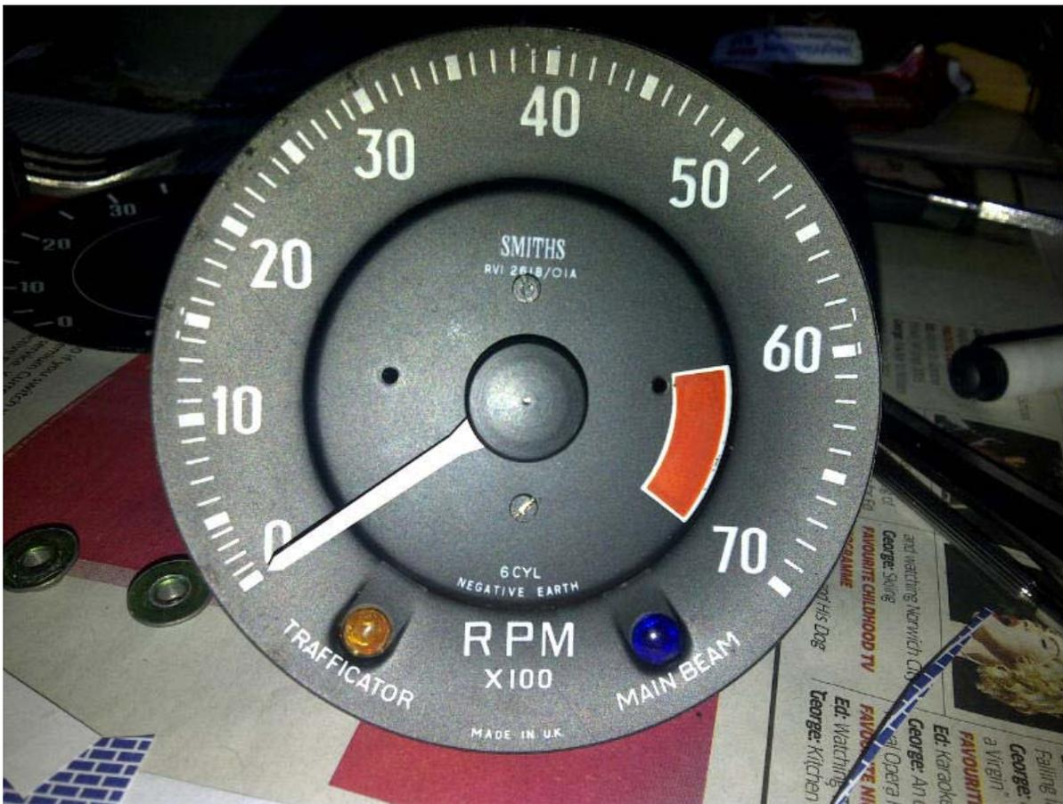
Now to fit it in the case - if you've done it right then the two light tunnels will line up, the electrical connectors poke out the back (you might need to relieve the case a little to provide some extra clearance) and the three screws will go in easily:
