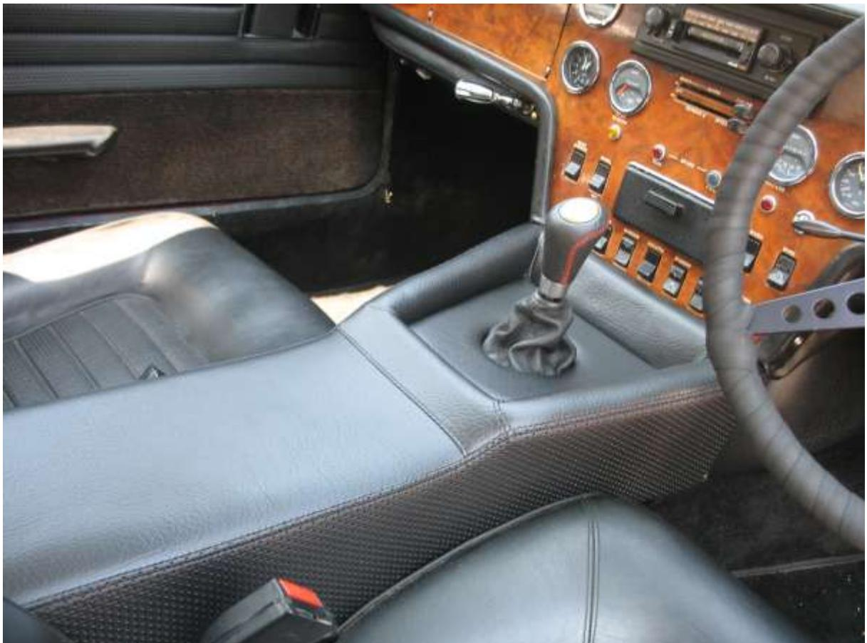
The tunnel top had been trimmed in matching black vinyl and basket wave with a new leather gaiter. The gaiter I used was an aftermarket item meant for a VW Passat. I turned up a black plastic ferrule to terminate the gaiter at the top of the gear lever.
