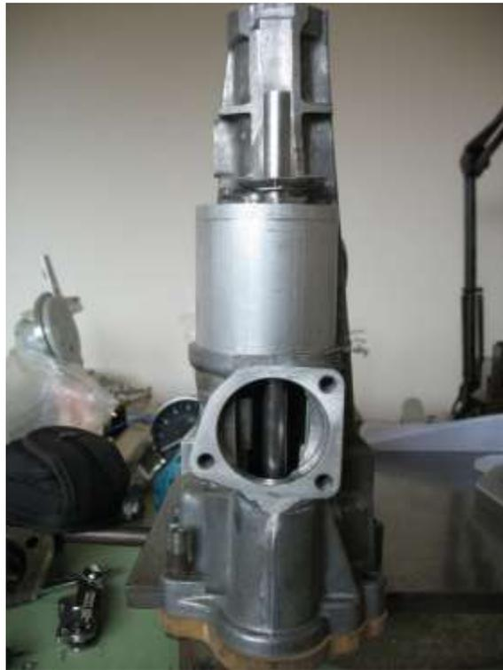
After welding I found the tail housing had distorted. The output shaft bearing was about 0.030" out of line with the output shaft. Fortunately it was only the bearing area that was seriously affected; the speedo drive for example still rotated smoothly.
