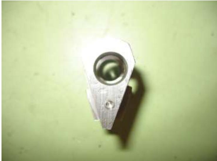
Having determined where the gear lever and bias mechanisms would be re-positioned I now had to modify the tail housing to provide a mounting platform and housing.
