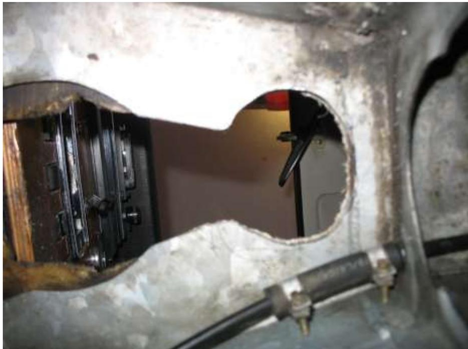
I closed off the old chassis aperture with a 0.070" thick reinforcing plate as shown in the photo below. This plate is bolted in place so it can be removed, particularly if I need to access the gear lever platform. This whole area will be insulated before the tunnel top is fitted.
