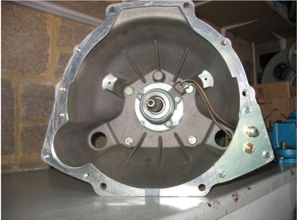
Taking note of one of the lotuselan.net contributors frustrating experience, I set up a test rig to ensure that the clutch did operate correctly before installing everything in the car.
