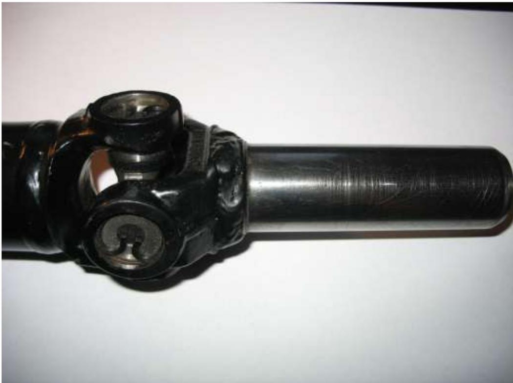
I have mentioned that the prop shaft needed to be a bit longer with the Type 9 installation, I had pinched a bit of length by repositioning the bearing in the tail housing but in case this was not enough I had made a short spacer which, if needed, would be sandwiched between the flanges at the diff end of the prop shaft. In practice I did not need to use this spacer, the prop shaft fitted fine without it.
