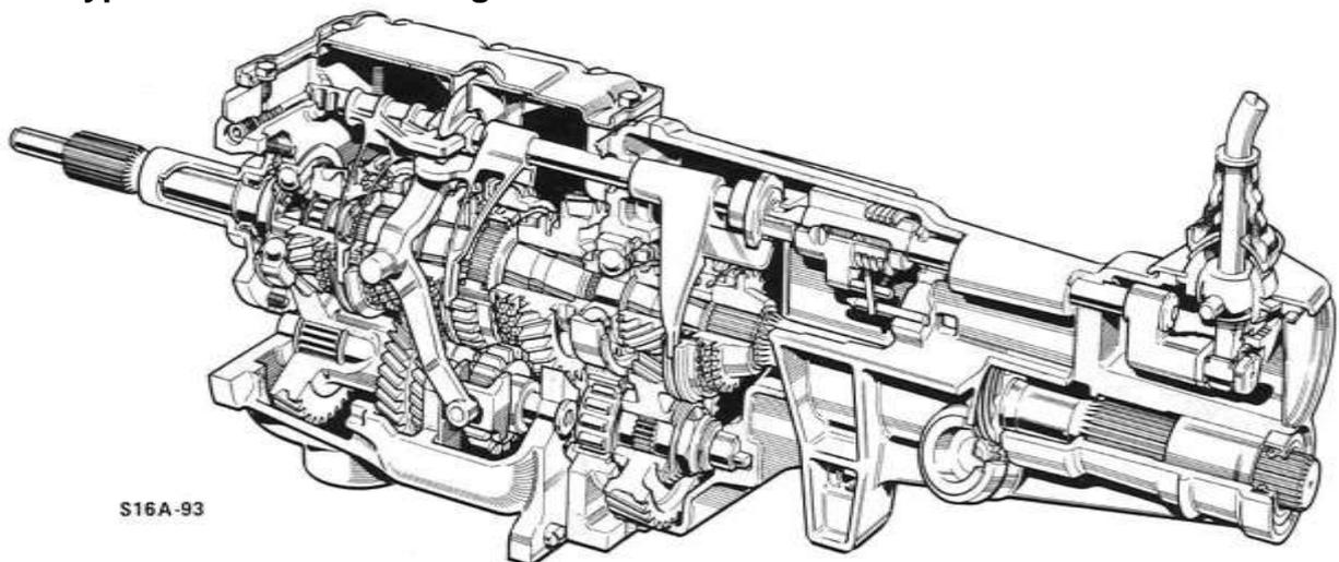
As you can see there is scope for re-positioning of the gear lever towards to the 5<sup>th</sup> gear cluster. Fortunately this is a single rail gear box so there is less to re-configure.
