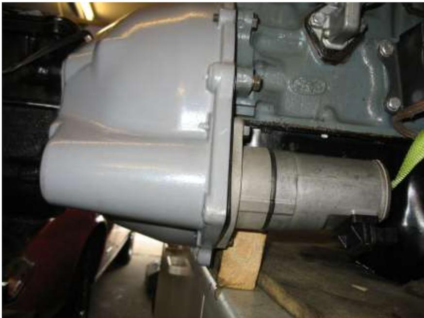
As with the tail housing this bell housing was thoroughly cleaned and powder coated mid-grey when I had finished the work on it.
