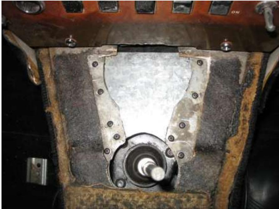
The photo below shows where the gear lever will sit in its new position. It puts the lever more or less in the centre of the platform on the tunnel top whereas the original 4 speed has the gear lever quite well forward, very close to the dashboard.
