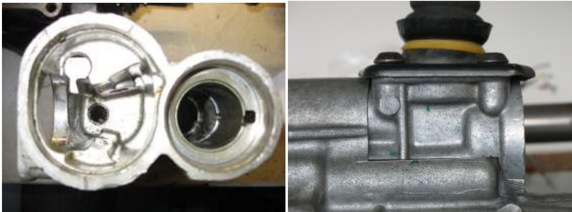
The photograph below shows the tail housing after welding on the gear lever platform.
