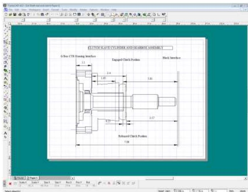
The above sketch shows the clutch layout I needed. But it also shows a single piece adaptor sandwiched between the slave cylinder and the front face of the gear box. I did not use this arrangement, in the end I modified the existing gear box input shaft bearing retainer and made a simpler spacer plate to finalise the position of the slave cylinder. I was also able to retain the existing input shaft seal in its original position in the retainer.
