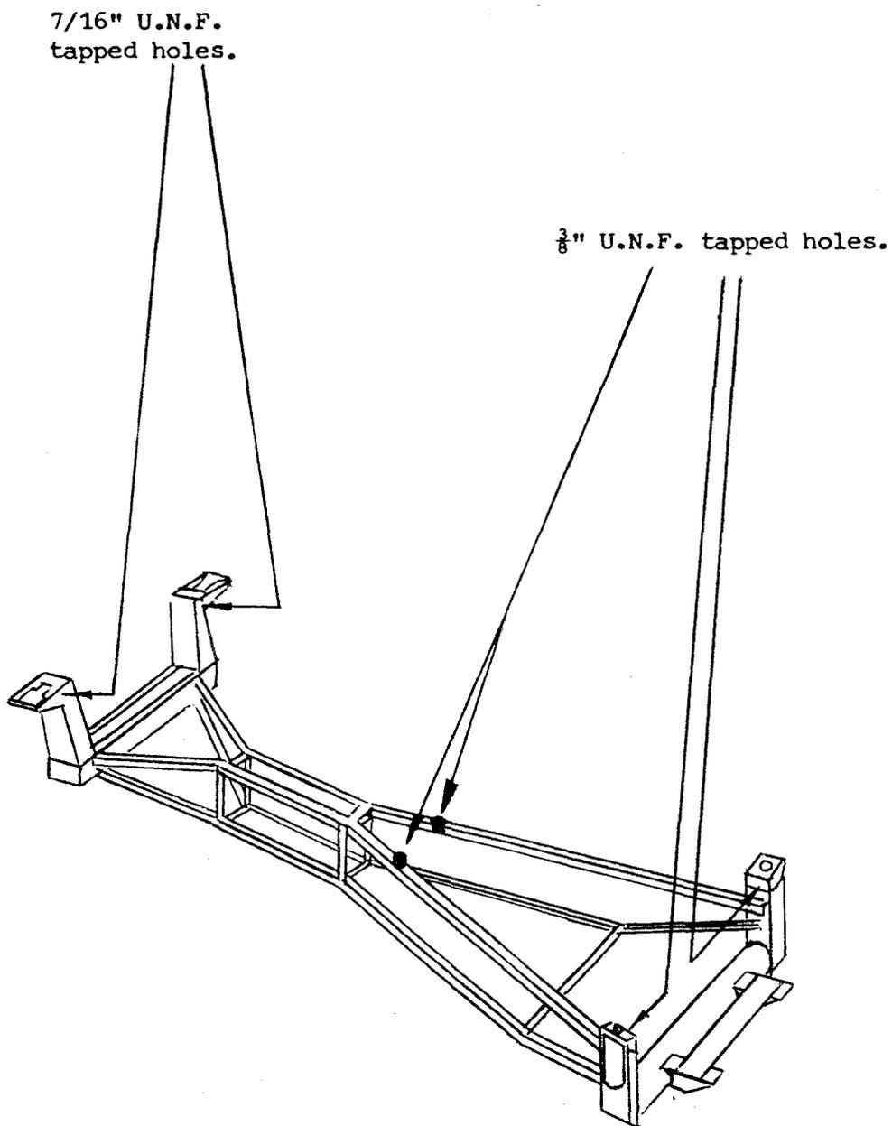
The six key body to chassis attachment points shown above are common to both stressed skin and spaceframe chassis.
