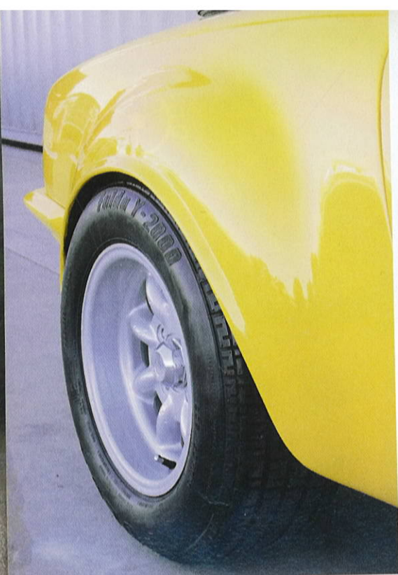
Flared arches accommodate 13x7 Minilites—standard Elan Sprint wheels were just 4.5 inches wide.
