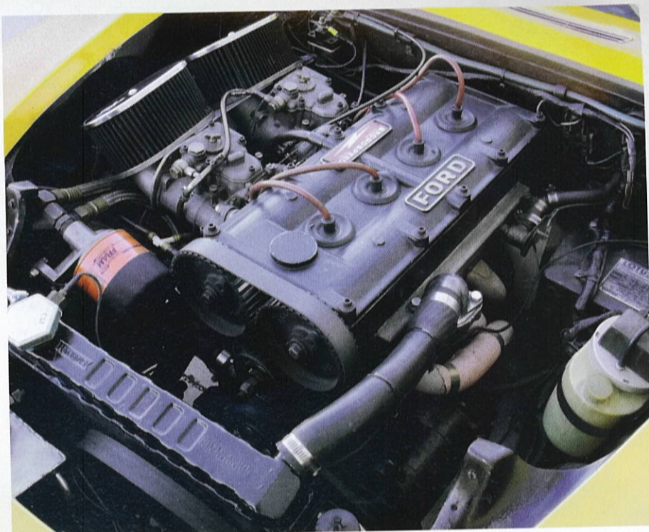
The 1600cc Formula Atlantic Cosworth BDA engine was capable of far more than its rated 170hp, but streetability demanded a more conservative power figure. Radiator had to be relocated to fit.
