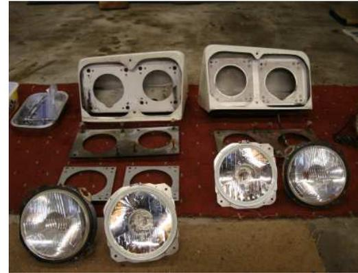
The outer bracket is a perfect fit. However the centre light bracket needs additional holes drilling to make fit for the S3's These also have a sprung screw which makes for easier headlamp adjusting.
