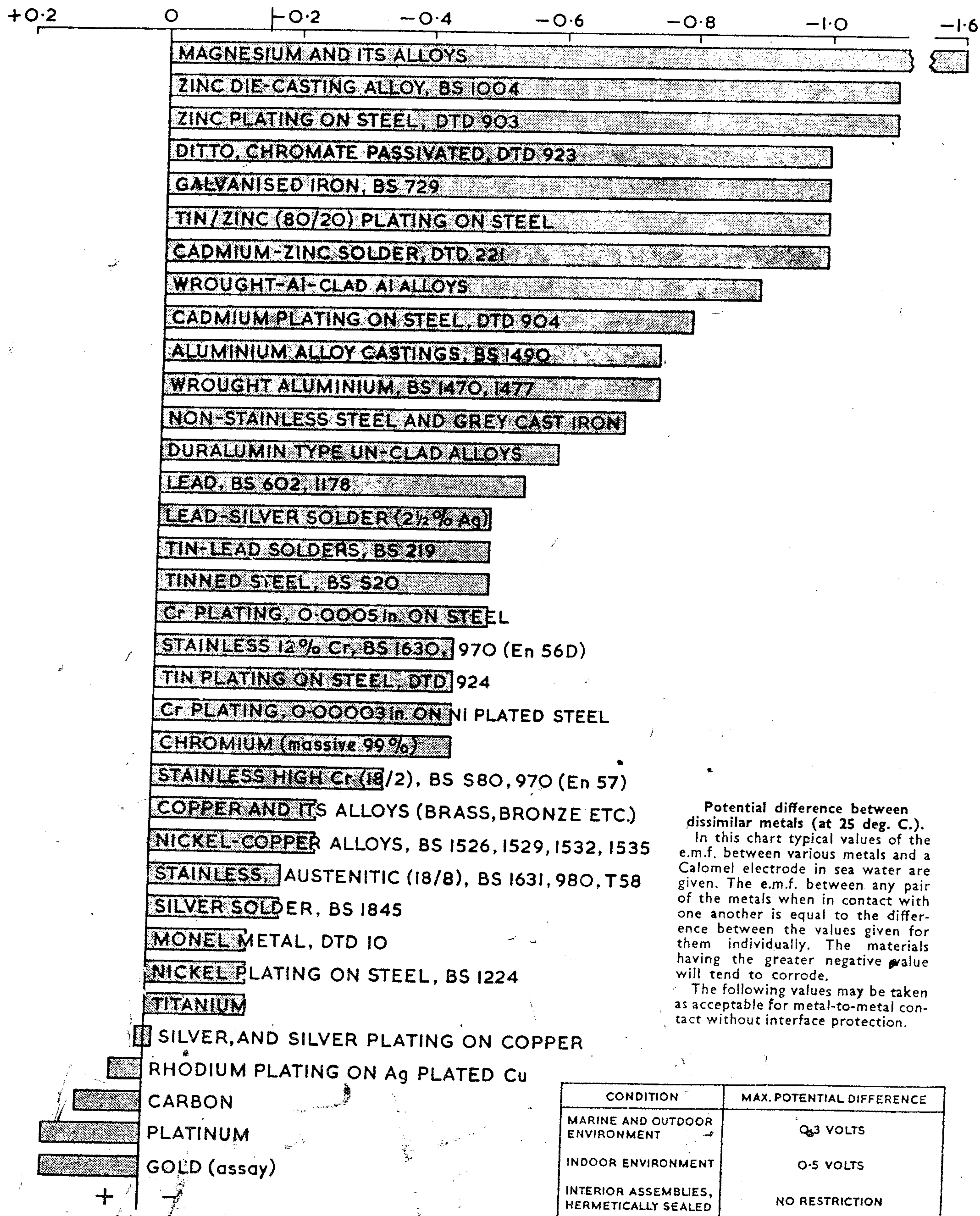
Potential difference between dissimilar metals (at 25 deg. C.).
